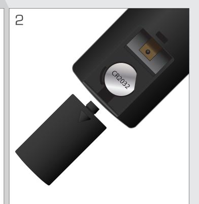
Replace the old battery with a new CR2032. Be sure that the + sign on the battery is facing up.
